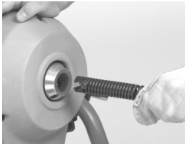
Figure 4 – Inserting Cable Into Front Of Machine
